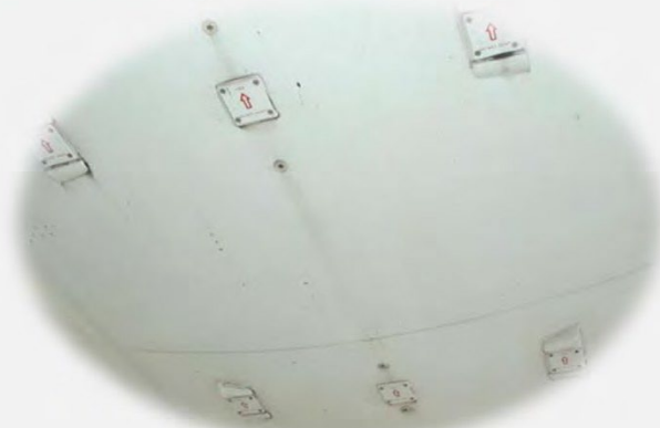
Radio Altimeter transmit/receiver antennas ..... Not damaged
