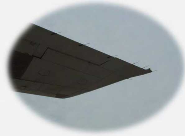
Static discharge wicks ..... NO MISSING PARTS AND NOT DAMAGED
