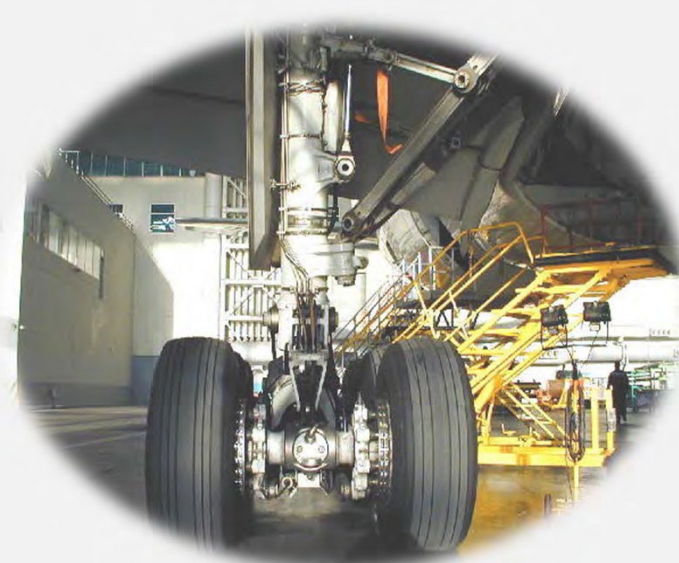
Wheel well .....Clear, not damaged, no missing parts and no fluid leaks
