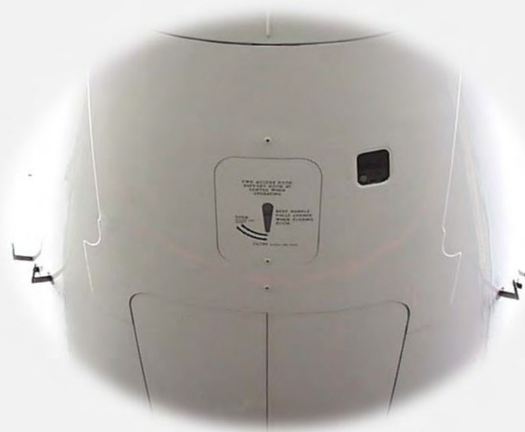
Forward access door.....Secure
