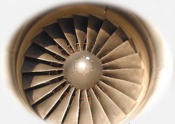
Fan blades, probes, and spinner ..... Clear, not damaged, no missing parts
