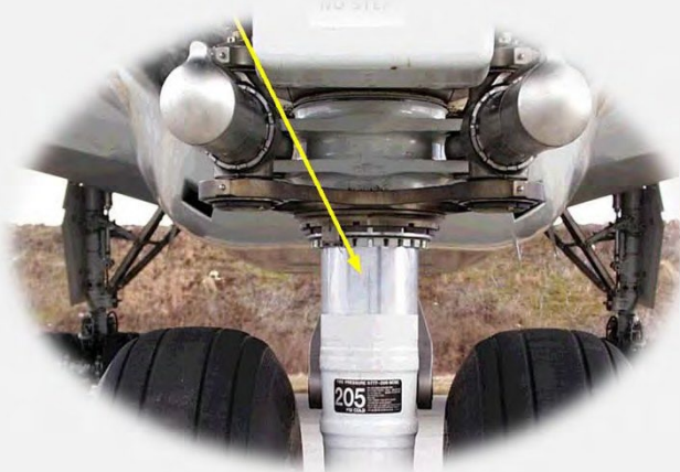
Gear strut .... NOT fully compressed ✓
