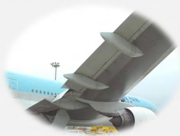
Aileron, flaperon, and trailing edge flaps ..... Clear, not damaged and no missing parts
